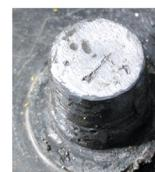
Reworked top of post. This indicate the hiding of abuse on the post and any rework marks will void the warranty.
