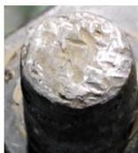
Indentations on the top of the post. This indicate "hammering" marks on the top of the post that can cause internal damage to the battery and reduce the lifespan of the battery.
