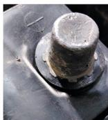
Excessive forces. It is visible from the battery casing that there has been excessive down force on the post that can damage the battery internally and reduce the lifespan of the battery.
