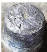
Post abuse marks. These marks indicate that the battery was not only used for automotive starting purposes as automotive battery terminals do not cause these marks under normal vehicle use.
