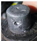
Hole drilled in post. This indicates that the battery was not only used for Automotive starting purposes and thus voids the conditions for warranty.
