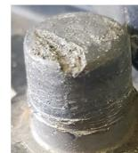
Lead melted away due to sudden excessive current on top of post (Arc marks). This may cause high internal current that may reduce the lifetime of the battery.
