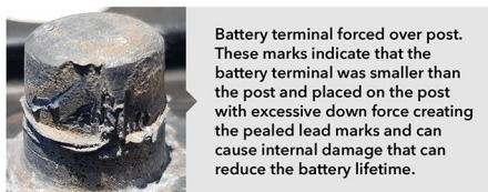
Battery terminal forced over post. These marks indicate that the battery terminal was smaller than the post and placed on the post with excessive down force creating the pealed lead marks and can cause internal damage that can reduce the battery lifetime.
