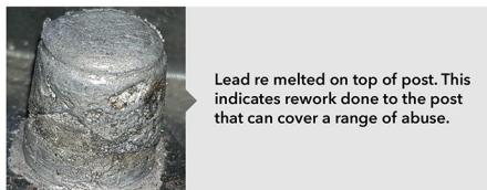
Lead re melted on top of post. This indicates rework done to the post that can cover a range of abuse.
