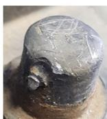
Missing lead from the post. This indicate excessive forces applied to the post that can cause internal failure and reduce the battery life.
