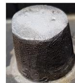
Reworked Post. The sharp edges and file/sanding marks on the top and sides of the post indicate that the post was reworked and tampered with this voids the warranty.
