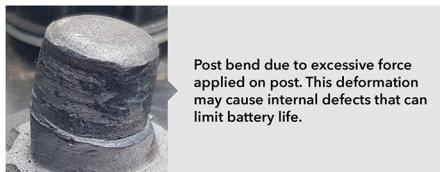
Post bend due to excessive force applied on post. This deformation may cause internal defects that can limit battery life.
