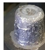
Excessive uneven marks on post. This indicate that the post was not only used for automotive starting purposes and thus voids the warranty.
